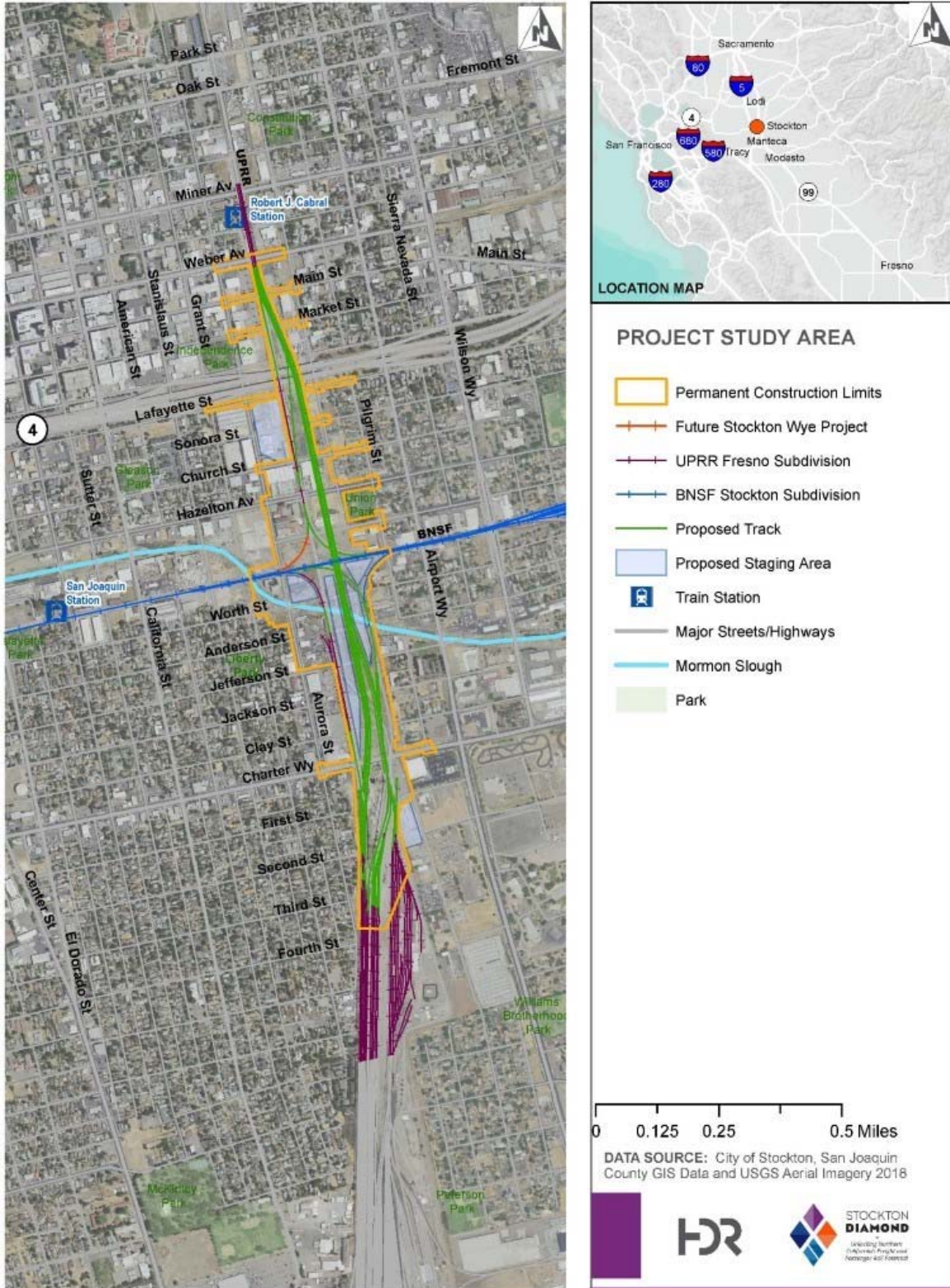
Figure 2. Proposed project area map for the new flyover structure path (green lines) and the existing railways supporting UPRR Fresno Subdivision service (purple lines) and BNSF Stockton Subdivision service (blue lines) over Mormon Slough in Stockton, California.
